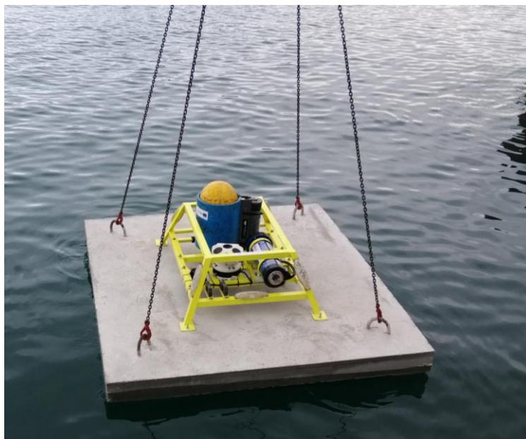
Figure 3. Detail of the anchoring system used.
